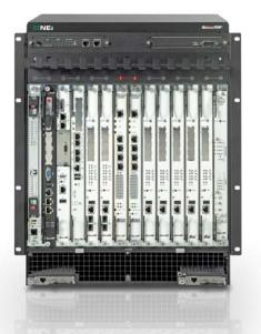
This 13U rack mount ATCA system packs 14 tool-less hot swap slots; two for dedicated fabric switch blades wired for either full mesh or dual star.
